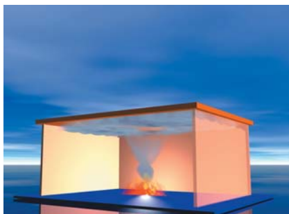
1. In the early stages, smoke from the fire will quickly rise into the roof space.
