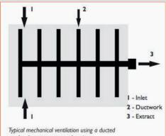
smoke clearance system: plan view
